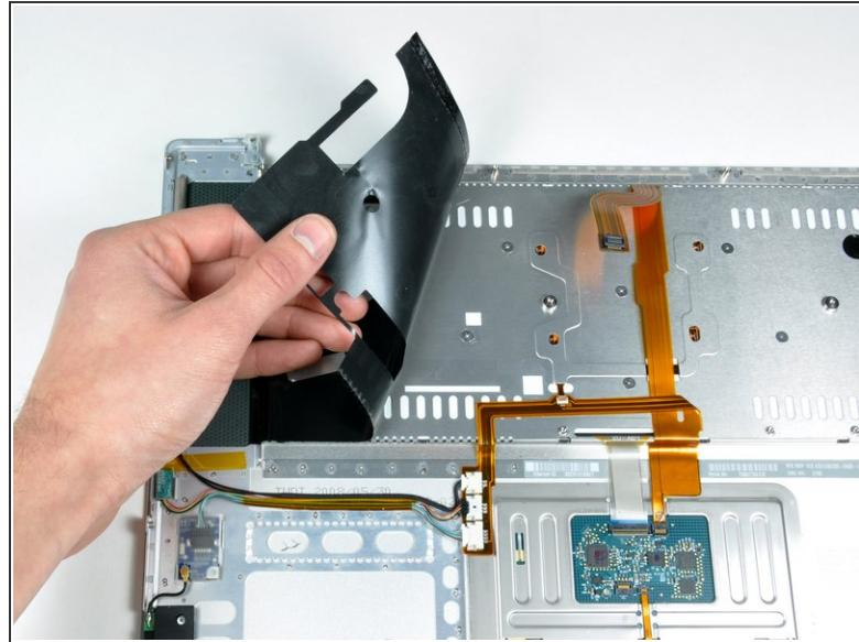
ⓘ In this step you will be peeling adhesive to give access to screws, it is not necessary to fully remove these shields.
